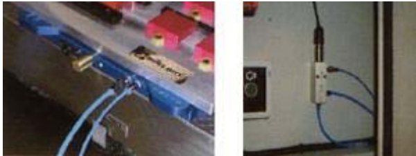
The small tube is connected to a low pressure safety switch to disable machine if air pressure is too low.
